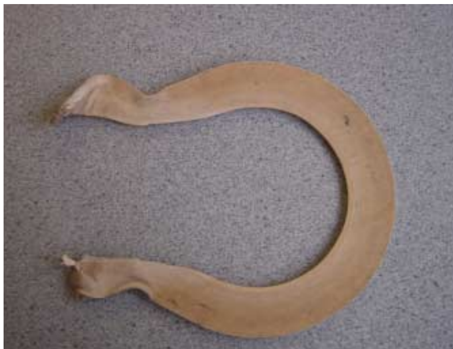
Photo 2 - Gasket after test 2 (with thermal cycle)
