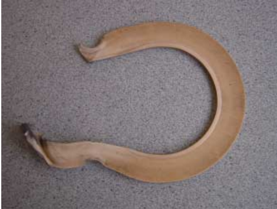
Photo 1 - Gasket after test 1 (without thermal cycle)
