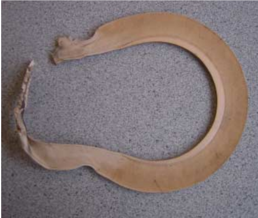
Photo 3 - Gasket after test 3 (with thermal cycle)
