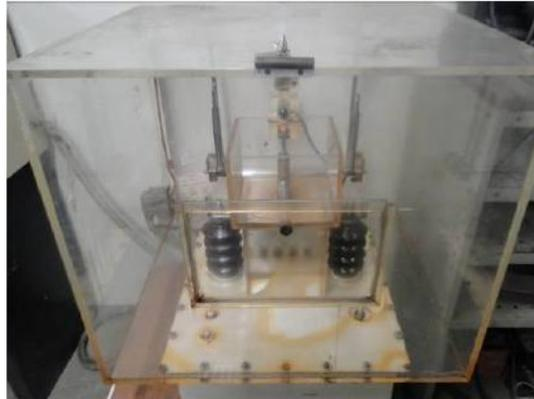
Figure 5 – Test rig for dielectric strength
