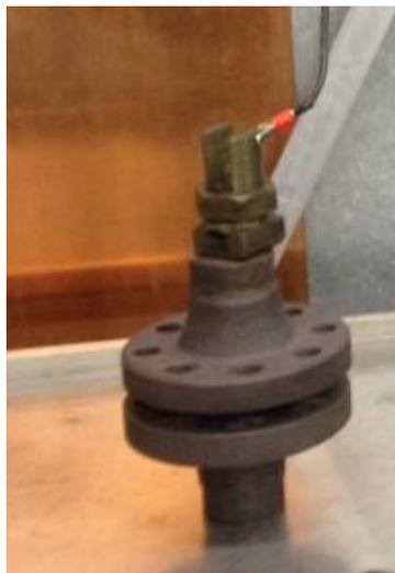
Figure 8 – Flanges without studs
