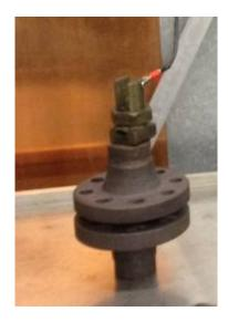
Figure 8 - Flanges without studs
