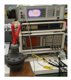
Figure 4 – Teraohmmeter
