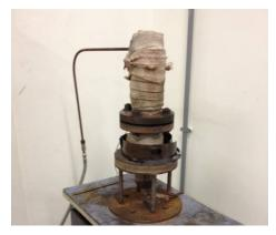
Figure 2 – Test rig for blow out
