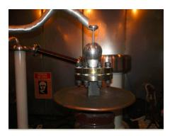
Figure 7 – Flanges with studs
