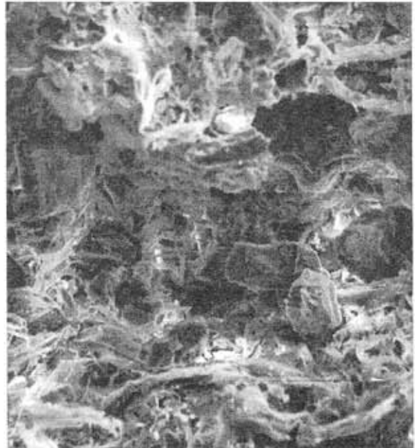
Figura 49 – rPTFE filled with Hollow Glass Micro-Spheres
