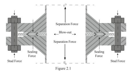
Initially, the Sealing Force is equal to the Stud Force. After pressuring the system, it is equal to the Stud Force minus the Separation Force.
