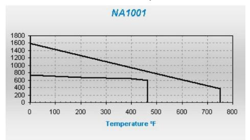
The P x T graph shown above indicates the service limits for this sheet considering pressure and temperature simultaneously...(Tests were performed with nitrogen on 1.6mm thick sheet). The "normal" curve represents the common usage area for this sheet while the "maximum" curve indicates the maximum limits. For applications near or above the "maximum" curve, contact TEADIT.
