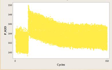
Style E-PTFE required a much higher initial torque to grant no visual leakage before test start – 42 lbf.ft
