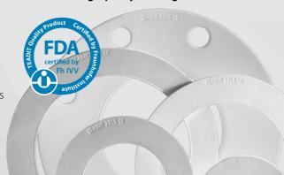
The inner bore of the 28 LS-LE gasket is enhanced with a diffusion barrier without any additional filler or other material, to avoid cross section leakage at low gasket stress. Therefore TEADIT® 28 LS-LE achieves high tightness with low bolt load.
