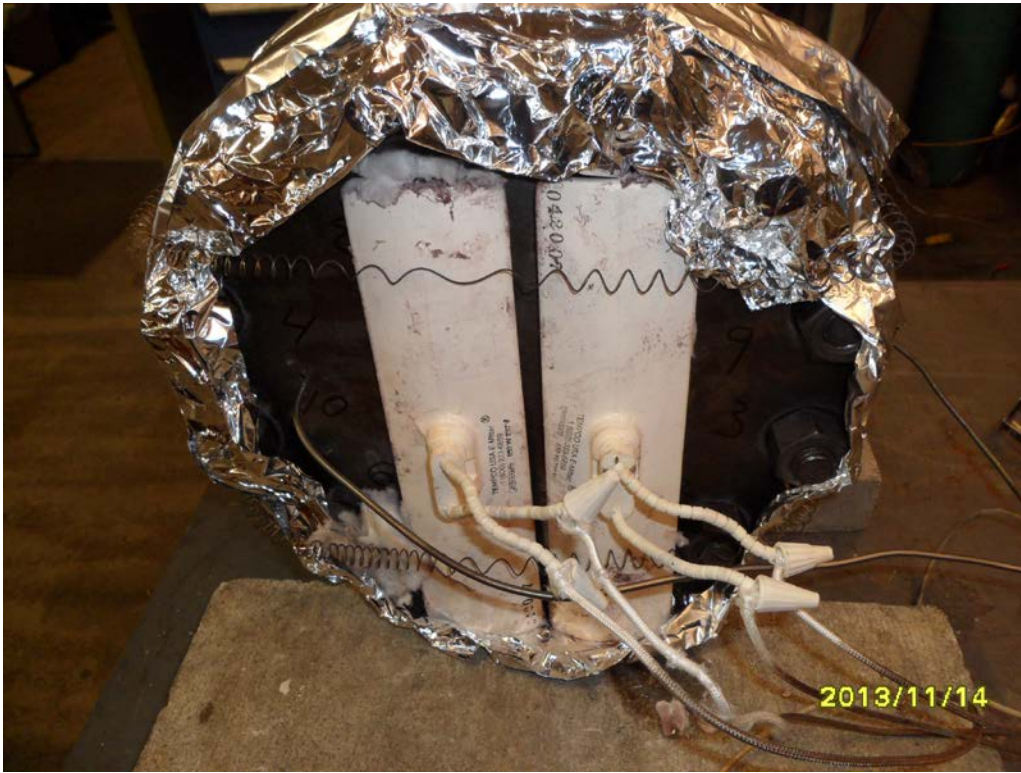
Test Gasket During Thermal Cycle
