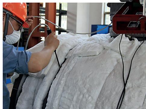
Over 20 years operation in line with Fugitive Emission Test Performed at 120°C, for SHELL project.
