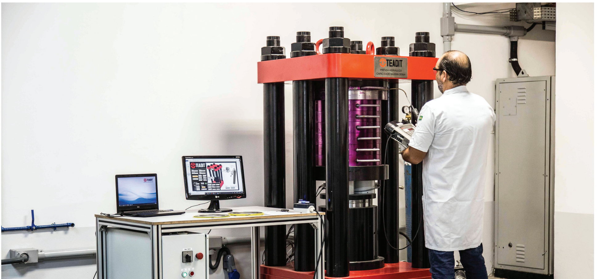
Teadit's cutting edge ASME B16.20 test rigs were specially designed to test spiral wound gasket performance.
