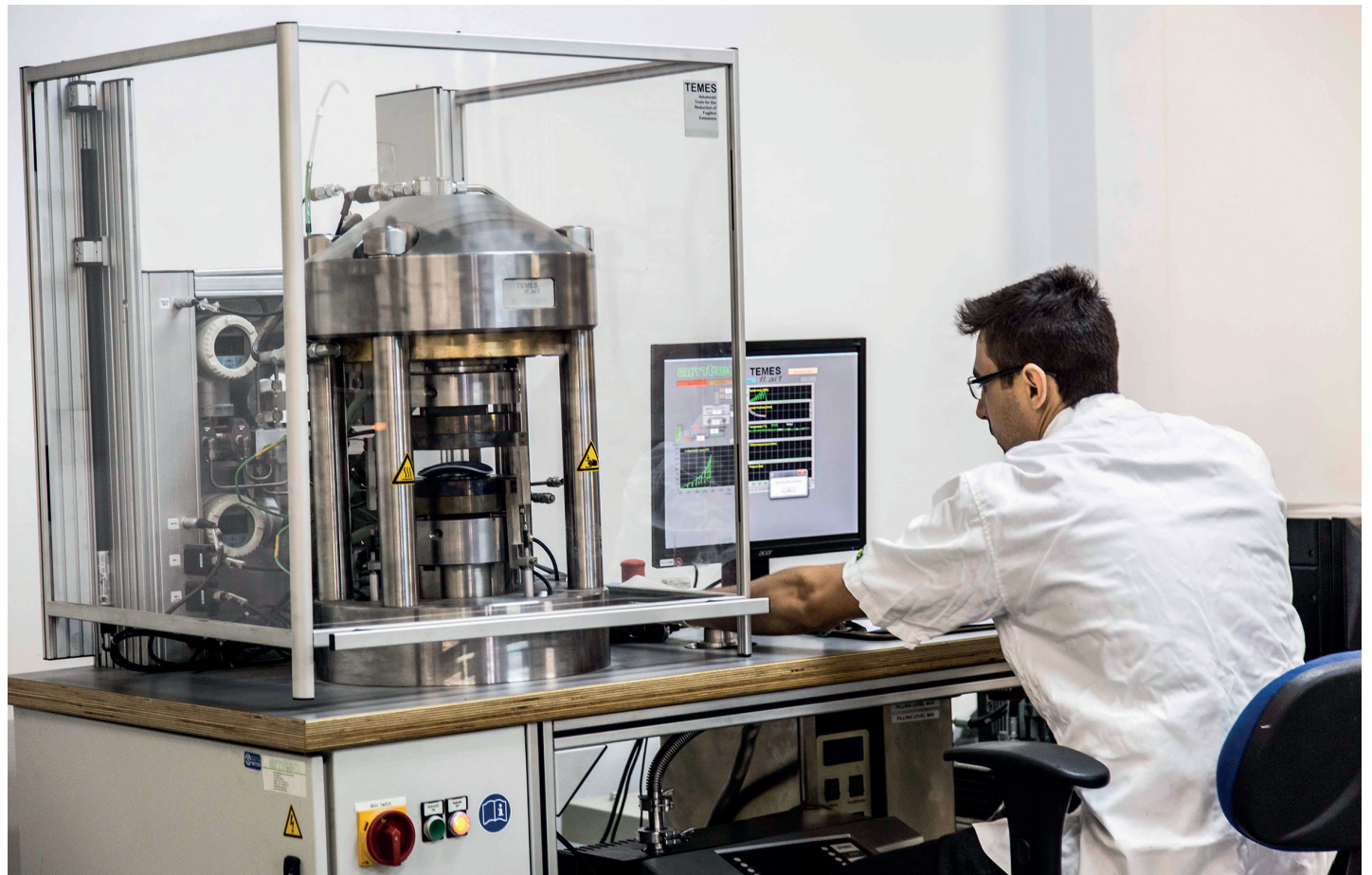
A TEMES "all-in-one" test rig can perform many standard gasket property and performance tests.
