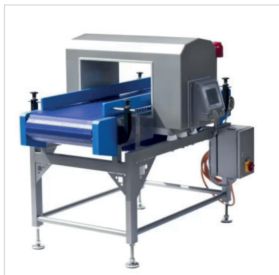
Highly sophisticated metal detection units can identify even trace amounts of detectable contaminants.
