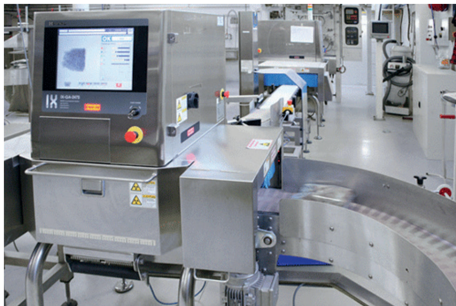
X-ray detection equipment is commonly used in food, beverage, and pharmaceutical applications.
