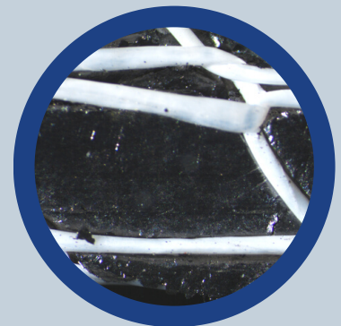
Close up of new polymeric structure in Teadit® 2848
