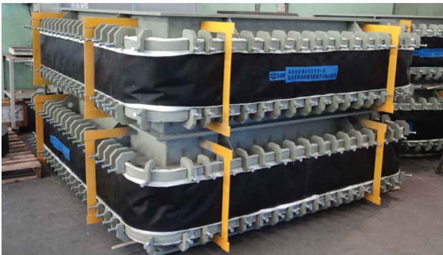
♣ Teadit fabric expansion joint: Made of reinforced fiberglass fabric and coated with PTFE to be used in a pelletizing plant.
