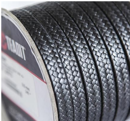
IMAGE 1: Expanded PTFE filled with graphite braided packing. This packing is made from expanded PTFE yarns with encapsulated particles of pure graphite and a high-temperature break-in lubricant. It is ideal for pumps and other rotative equipment with higher surface speeds and temperatures than those that can be typically handled by pure PTFE packing styles. (Images courtesy of Teadit)
