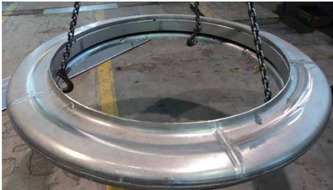
➤ Heavy wall bellows, manufactured for use in a fertilizer plant. Image courtesy of Teadit.
