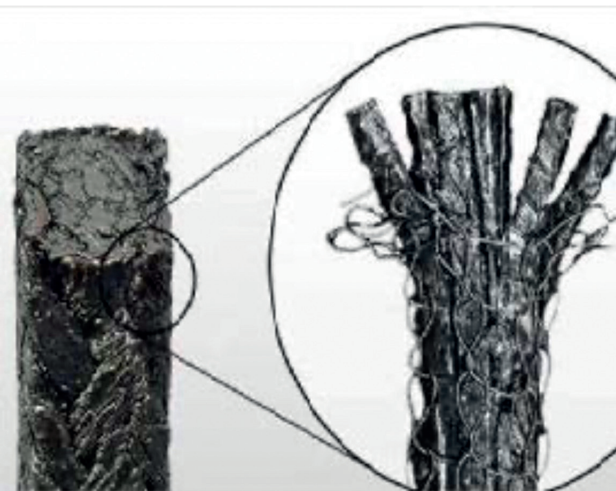
Close-up view of Teadit's 2235 style packing. It is fabricated with individual strands of graphite tape reinforced with an Inconel wire.
