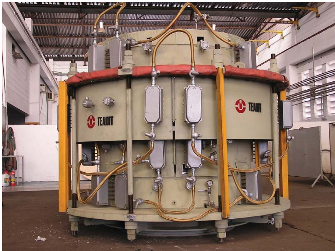
➤ An in-line pressure balanced expansion joint with a heating system to maintain the bellows temperature in a specific range.
