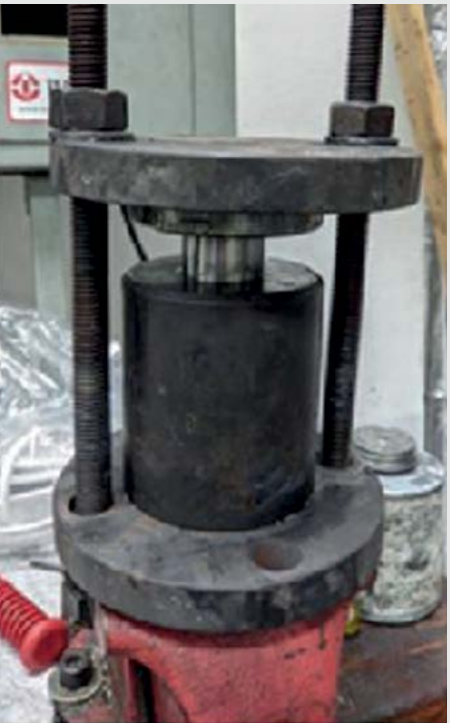
Figure 4: Stuffing Box Testing Rig used for oxidation simulations.
