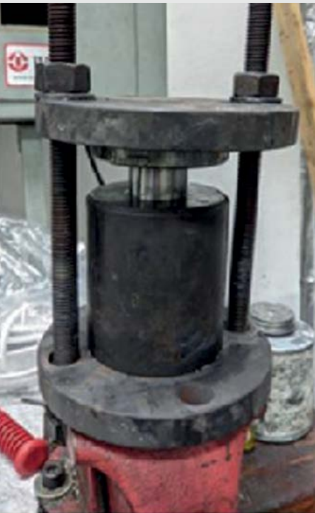
Figure 4: Stuffing Box Testing Rig used for oxidation simulations.
