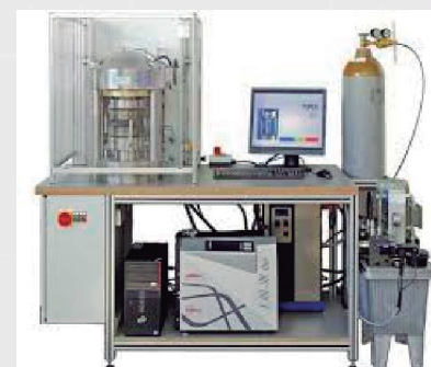
Pictured left to right: Leakage performance curve of the TEADIT® 24 SH gasket under 40 bar hydrogen. The TEMESfl.ai test bench is used to test the sealability of gaskets with hydrogen. This is an example of how TEADIT® tests a gasket to understand its performance when sealing hydrogen.
