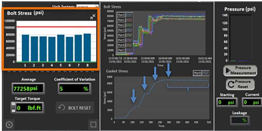
IMAGE 2: Software interface. The test rig used for the study is shown in Image 1 and consists of two ASME B16.5 NPS 4-inch blind flanges, pressure class 150, equipped with eight 5/8-inch bolts instrumented with strain gauges to measure the bolt stress over time. The material for the flange is ASTM A105, and for the bolts it is SAE Grade (tensile strength of 180 kilopounds per square inch [ksi]). The top flange has a hole leading to an internal chamber, which can be pressurized. For this research, this feature was not used.
