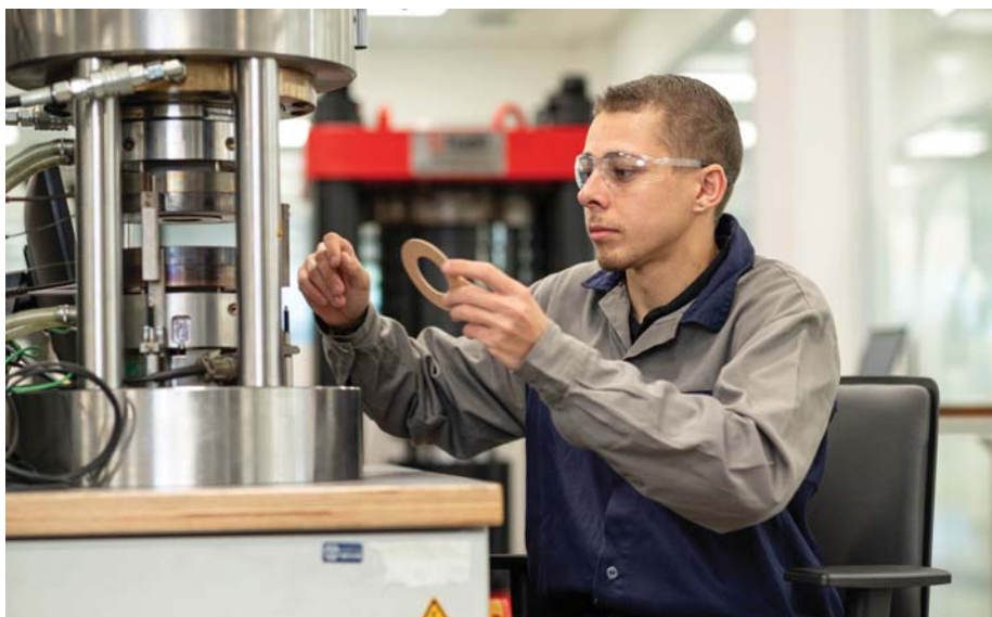
A subject matter expert at TEADIT's innovation hub installing a cut gasket in the hydraulic press for testing.
