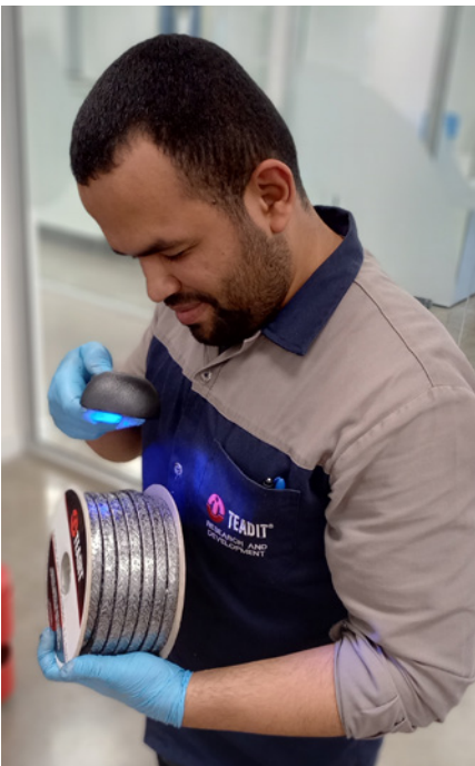
Figure 1: Depiction of engineer viewing TEADIT® 2848 packing with TEADIT® TAGS™. TEADIT® TAGS™ are traceable particles that may have different forms, compositions, sizes, and are able to be detected by distinct apparatus. This groundbreaking design ensures the traceability of the product before, or even after, it has been in service.
