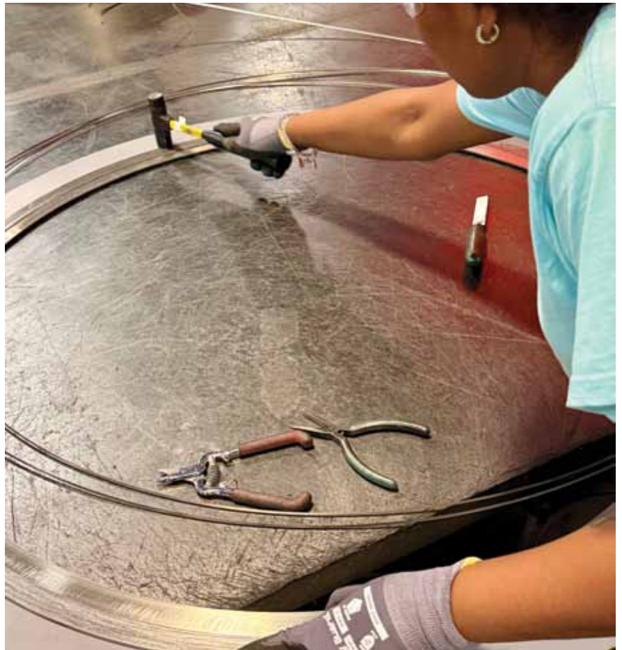
≈ TEADIT® sealing experts engineering a metallic kammprofile gasket.
