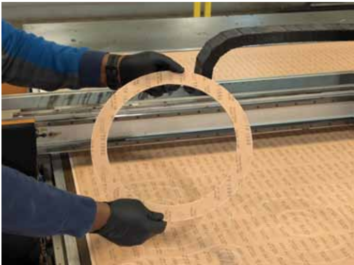
➤ A depiction of the fabrication process for TEADIT®'s TF1590 gasket solution.
